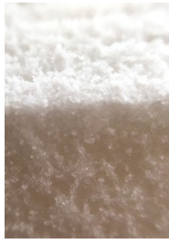
Macro view of SLS 'Orange peel' effect
