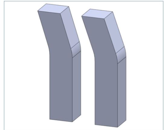
*Example of warping on a tall, thin part without support structures*
