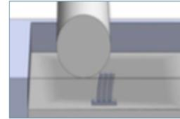
Force from the roller may cause tall, narrow parts to shift in the build
