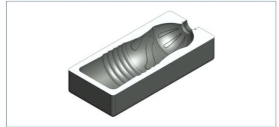
*Reduce mass built in DMLS to reduce cost*
