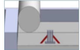
Support structures prevent parts from shifting in the build
