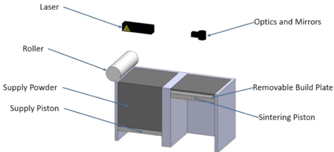
*Typical components of a DMLS machine*
