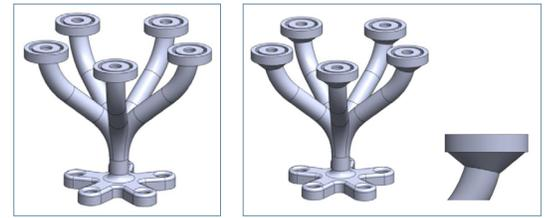
*Add chamfers or fillets to overhanging geometry to make it self-supporting*
