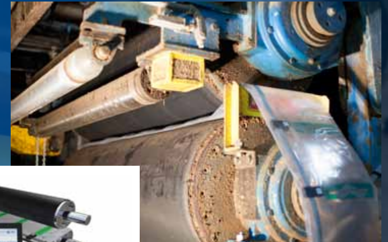
FIGURE 5 THE NPAT PRESSURE MAPPING SYSTEM (POSITIONED BETWEEN THE ROLLERS ABOVE) HELPS TECHNICIANS ESTABLISH A “GOLD STANDARD” ROLL ALIGNMENT SETTING.
