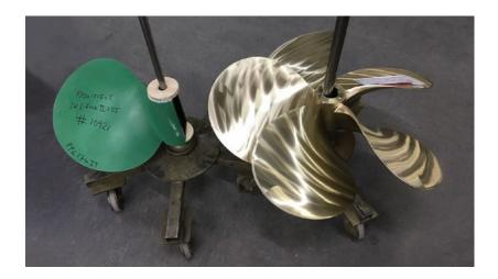
A typical pattern print for a 750mm long design takes just 40 hours to print. Total production time is just 48 hours when including post-processing work. That two days means a 33% faster pattern production time, cut down from three days. A 90% reduction in pattern maker costs further highlights the benefits of bringing large-format 3D printing in-house.
